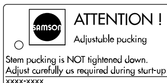
Fig. 3: Label when an adjustable packing is installed
